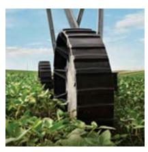
NFTrax's unique design controls water runoff and reduces track erosion for faster field drying time.
