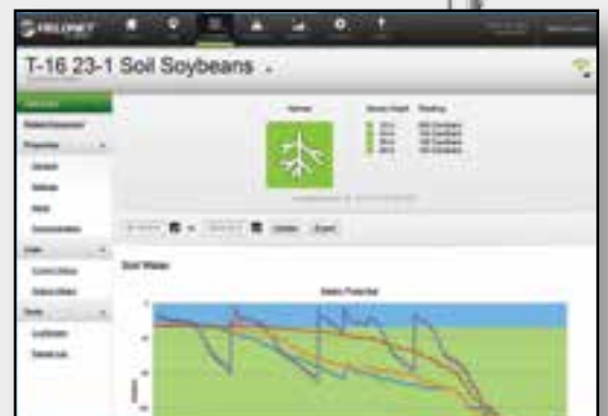
FieldNET provides graphing and configuration to monitor soil moisture status.
