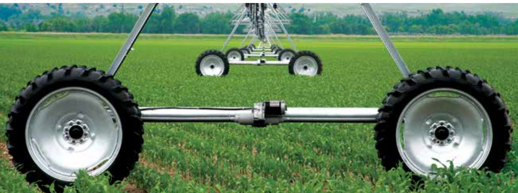
Zimmatic pivot with 43 rpm motor
