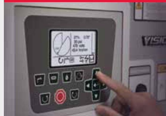
A graphical backlit display provides effortless operation, even at night.
