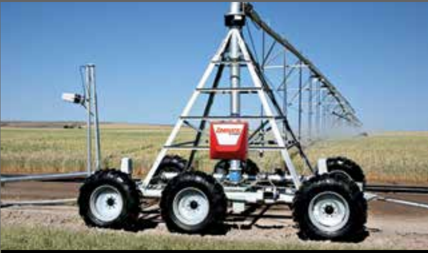
Six-wheel high traction platform
